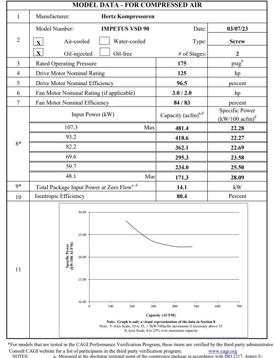
a. Measured at the discharge terminal point of the compressor package in accordance with ISO 1217, Annex E; ACFM is actual cubic feet per minute at inlet conditions.
